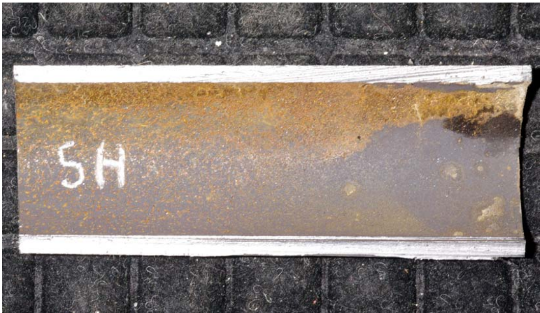
FIGURE 40. Superheater tube sample (from the furnace) interior.
