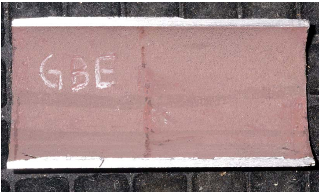
FIGURE 44. East generating bank tube sample interior.
