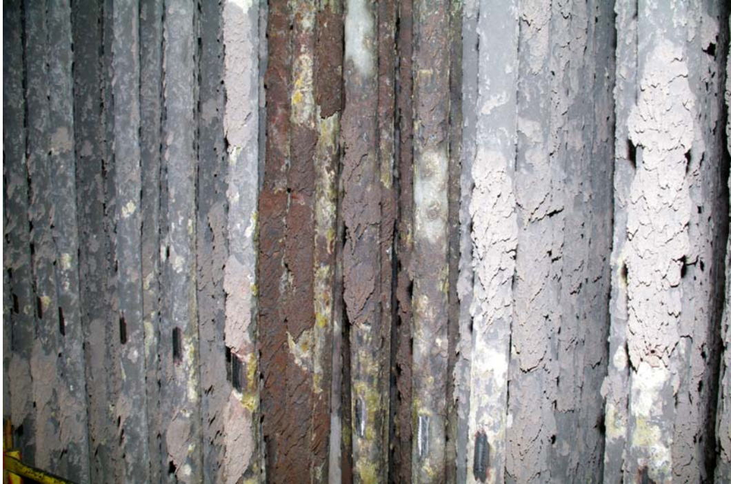
FIGURE 16. Superheater tubing from the furnace (center discolored tubes from leakage above during tubing removal in penthouse).
