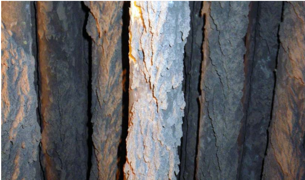
FIGURE 17. Another view of the superheater pendants, note lack of separation.
