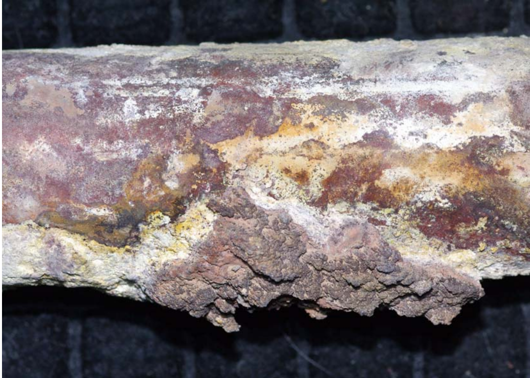
FIGURE 39. Close-up view of the superheater tube sample exterior (from furnace).
