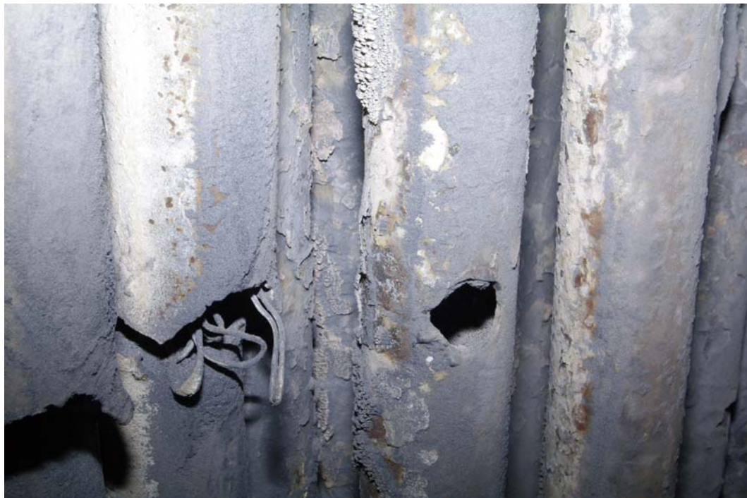
FIGURE 26. Generating bank tube failures.
