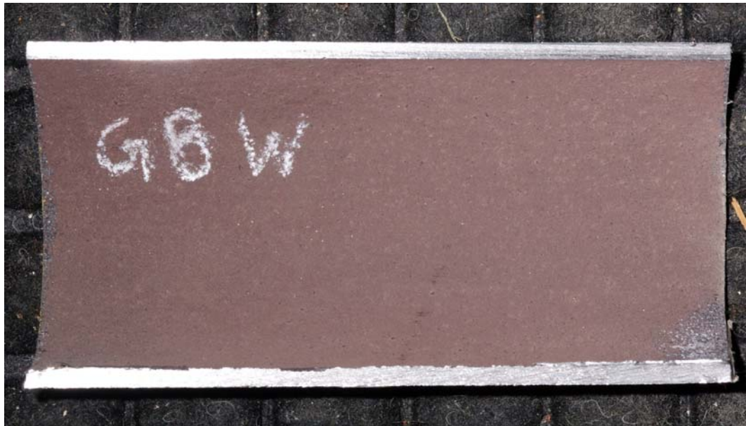
FIGURE 46. West generating bank tube sample interior.
