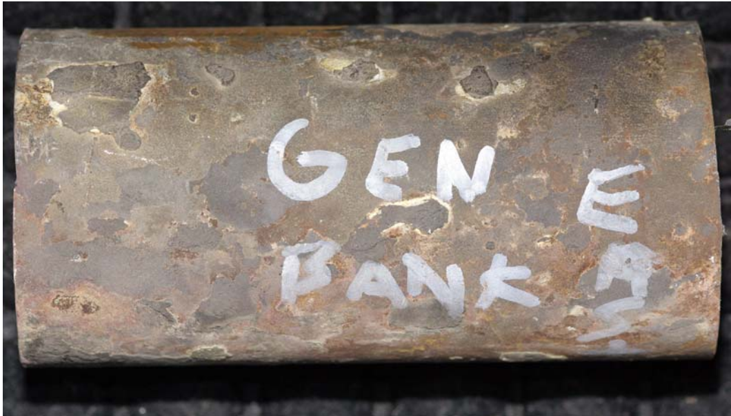
FIGURE 43. Generating bank tube sample from the east side.
