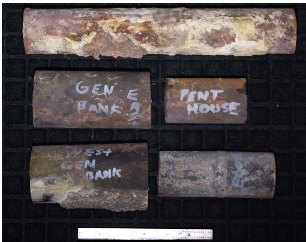
FIGURE 38. Tubing samples after removal (top sample is superheater from furnace).
