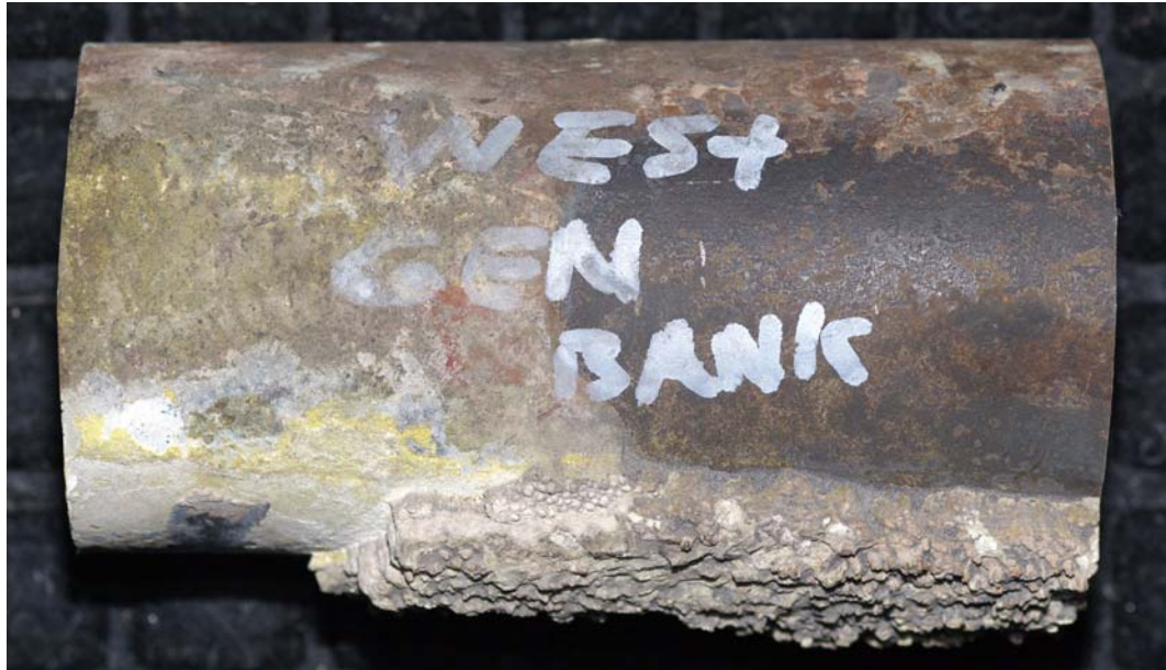
FIGURE 45. Generating bank tube sample from the west side.
