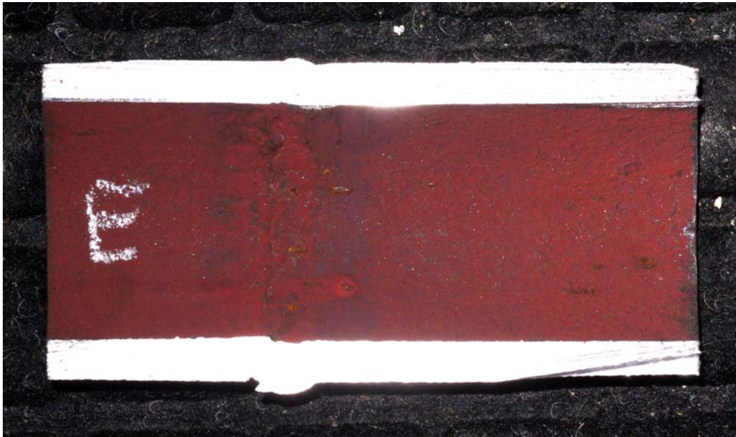
FIGURE 48. Economizer tube sample interior.
