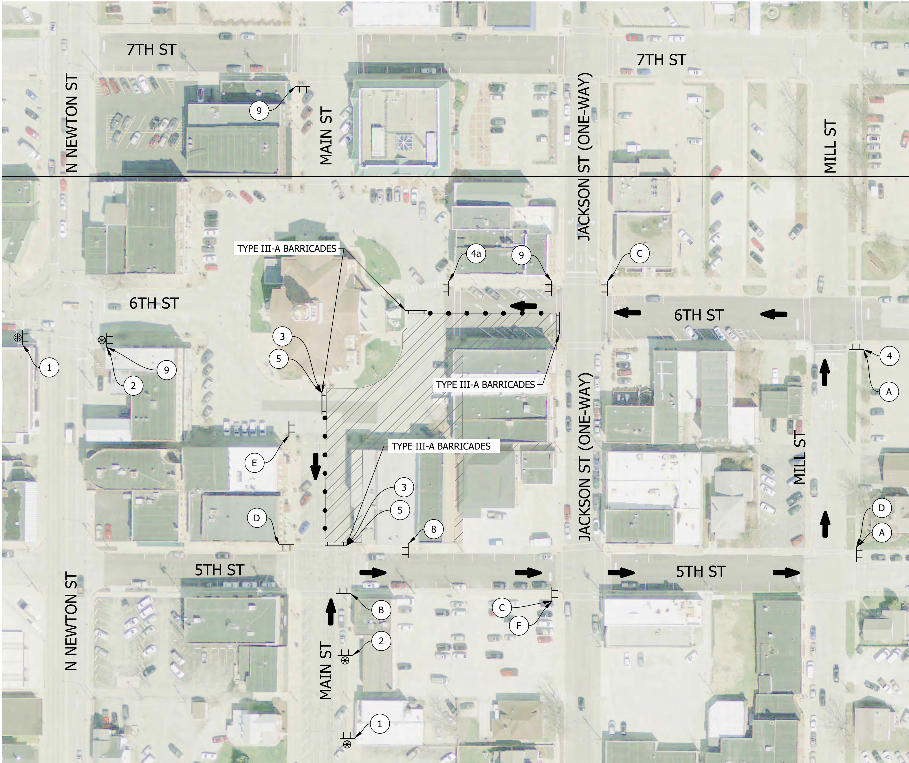
Detour Route "North Main/East 6th" Phase III
